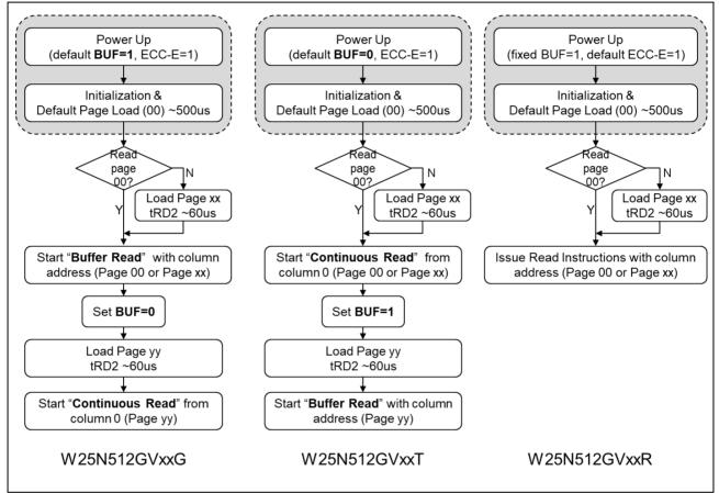
Figure 3. W25N512GV Flash Memory Operation Diagram
