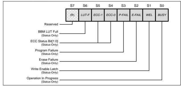
Figure 4c. Status Register-3 (Address Cxh)
