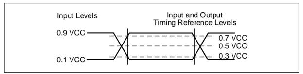
Figure 34. AC Measurement I/O Waveform
