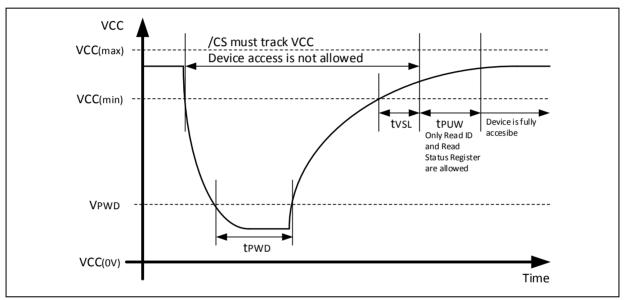
Figure 33a. Power-up Power-down Timing and Voltage Levels
