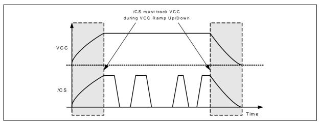
Figure 33b. Power-up, Power-Down Requirement
