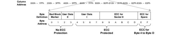
Figure 2. W25N512GV Flash Memory Architecture and Addressing
